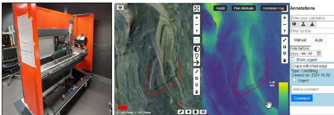
Figure 1: Condition Assessment Scanner (CAS) and CAS data visualization platform
